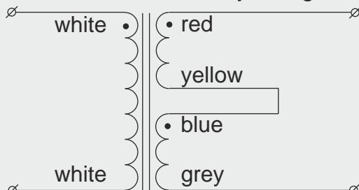
parallel operation to double the secondary current
