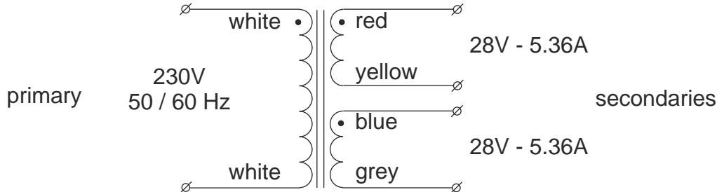
serial operation to double the secondary voltage
