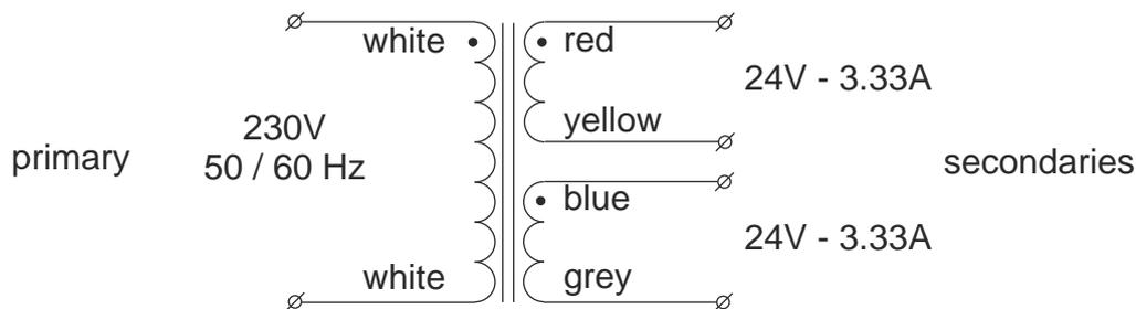
serial operation to double the secondary voltage
