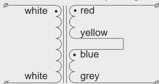
parallel operation to double the secondary current
