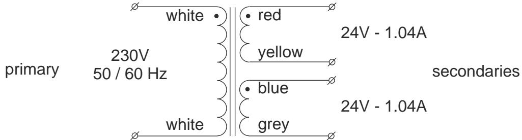
serial operation to double the secondary voltage
