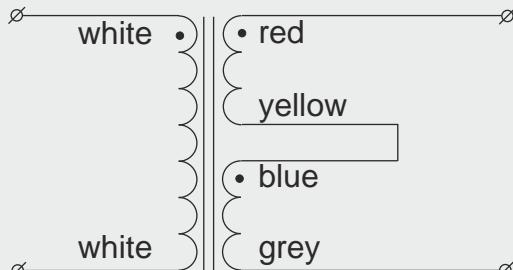
parallel operation to double the secondary current
