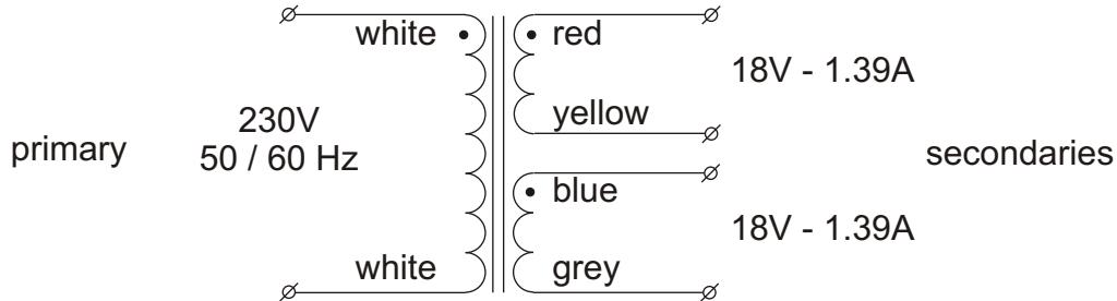
serial operation to double the secondary voltage
