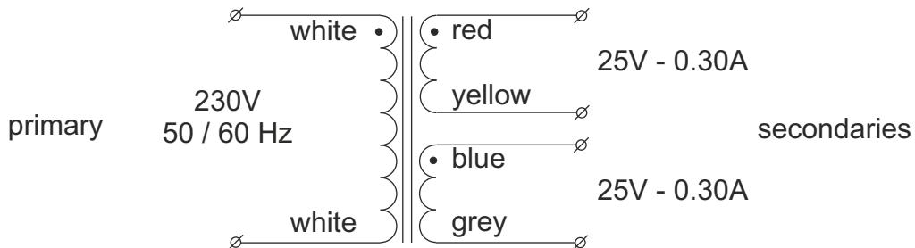
serial operation to double the secondary voltage
